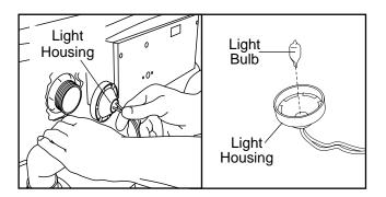
To replace the light bulb, pull the old bulb out of the housing and insert a new light bulb. Re-attach the light housing to the spa shell. Re-attach the access cover to the spa unit.
